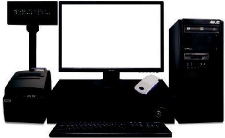
**PM-900TEN Cashier Station** is used for central payment application - it reads the data encoded in a barcode ticket received; calculates and displays the required amount of parking fee on the fee display. Once a payment is made, a new barcode with payment completed data is printed on the same ticket for exit validation at any exit terminal
